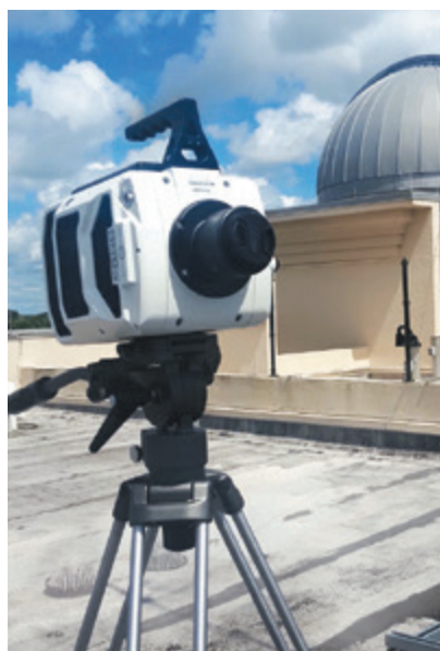
Phantom v1210 digital ultrahigh-speed camera.
